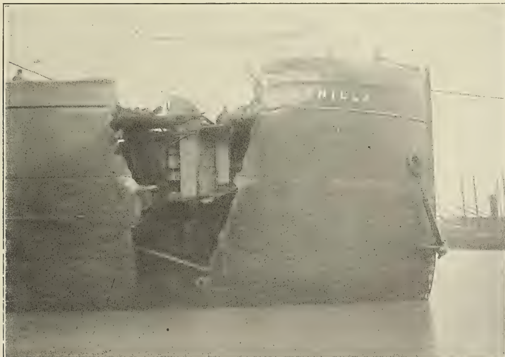
THE HOLE CUT IN THE SIDE OF THE STEAMER CORONILLA BY THE JAMES JOICEY.
